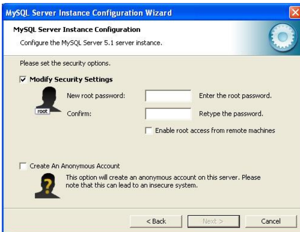
Figure 5. MySQL security settings. This is the most critical part of the installation because you need to remember the password that you enter.
