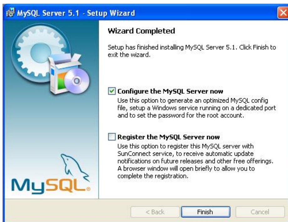
Figure 1. Last stage of MySQL installation dialog. Select “Configure the MySQL Server now” and click on “Finish” to launch the MySQL Server Instance Config Wizard. Registration of the MySQL server is unnecessary.
