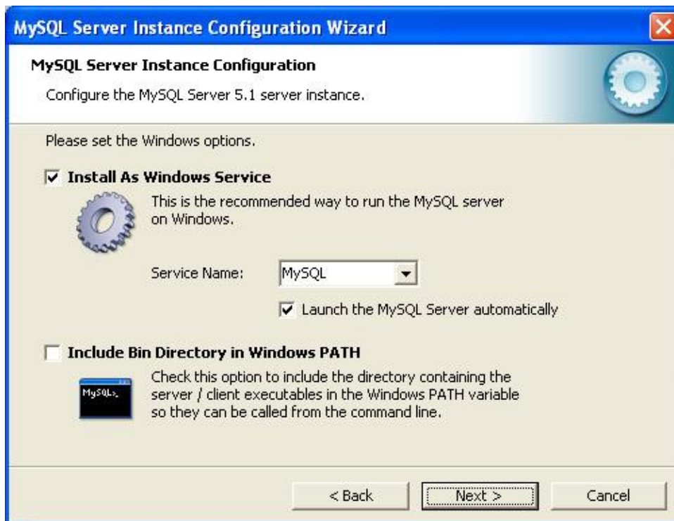
Figure 4. Install MySQL as a Windows service. SpikeStream does not need the MySQL bin directory to be included in the Windows PATH, but it will not create any problems if you select this option.
